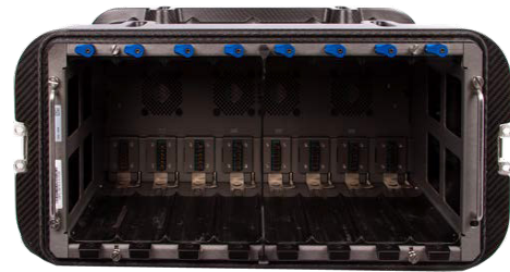
Figure 1: Front of Voyager 8 PLUS Showing 8 Voyager Module Slots
